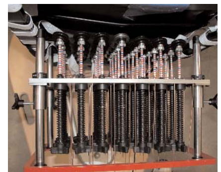
Figure 3. Overhead views showing all diodes in the fully extended position (above) and the fully retracted position (below).
