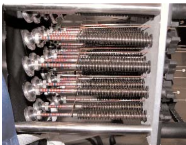
Figure 2. Side view of thirty-five spring-loaded diodes.
